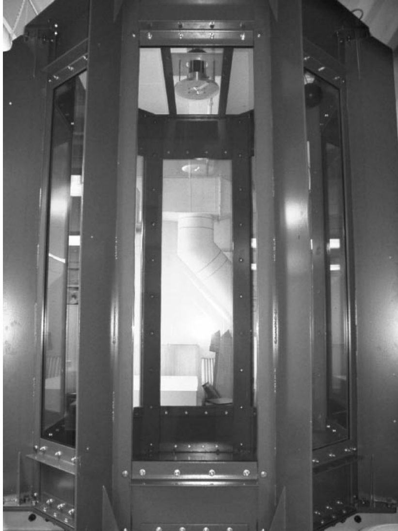
FIGURE 1. Side view of the facility designed, constructed and operated for the present experiments that enabled \sim 1000^3 whole-field concentration measurements above the mixing transition. The octagonal tank provides four pairs of vertical windows at right angles to each other that facilitate non-intrusive optical imaging of the flow. The tank has an internal diameter of 6 ft, an internal height of 9 ft, and a capacity of 8 tons of water. A jet seeded with dilute aqueous disodium fluorescein dye was generated in a blow-down manner and issued through a nozzle of exit diameter d = 2.54 mm machined flush with the base plate of the plenum, visible at the top. The jet was directed downwards at a Reynolds number of Re \sim 20\,000 with a Schmidt number of Sc \sim 2000 . Imaging was conducted in the far field of the flow at a downstream distance of z/d \sim 500 nozzle diameters and the large-scale transverse extent of the flow at the imaging location was \delta \sim 0.5 m.
